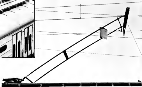
Two views of the remote-control pan trolley developed so that one-man cars could operate, without stopping, between sections of line powered by third rail and overhead trolley. Note airfoil below collector shoe, which serves to maintain pressure against trolley wire needed to collect current at speed.
